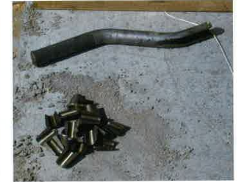
(c) Implement used to hammer the wedges into position (P439)
