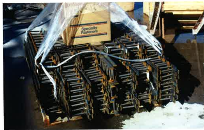
(a) Stud rails reinforcement (P411)
