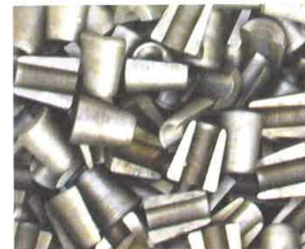
(a) Wedges are used to anchor strands (P437)
