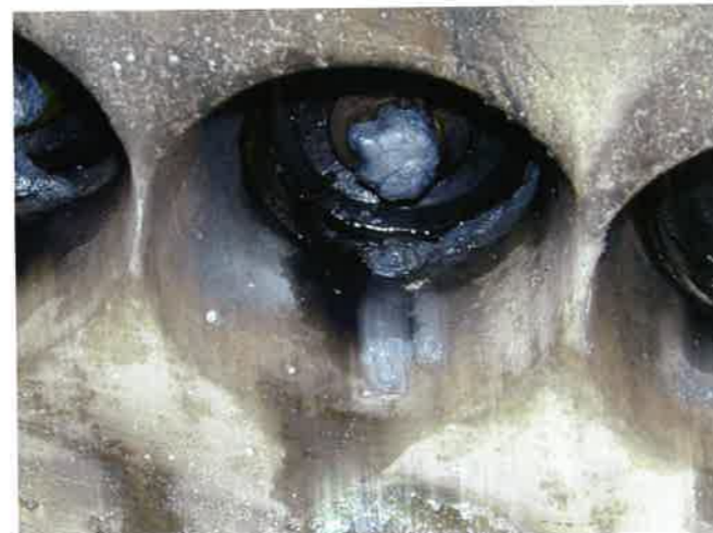
(b) Flame-cut fused strand end (P450)
