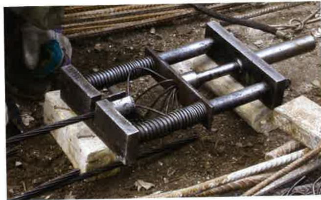
Figure 2.5.2A-7 Device Used to Form Onion-Shaped Dead Ends (P511)
