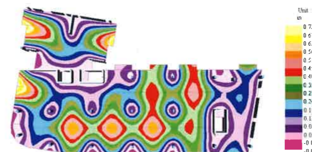
FIGURE 4.10.6.4E-2 Deflection Contour of the Floor System under Combined Actions of Dead and Live Loads (P256a, P256b)
